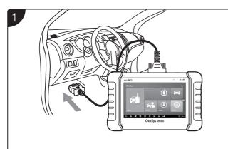
• Connect the vehicle and the key programming tool with the supplied main cable.
